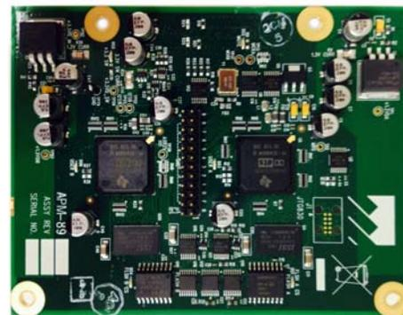
Momentum Data Systems APM modules are a superset of MDS' DAE modules, adding an integral ARM-based processor running Linux to create a stand-alone subsystem compared to the DSP-only DAE modules.
